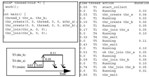
Figure 2: An example program and the output from the Recorder. The operating system assigns the following thread identity numbers to the threads: main = 1, thr\_a = 4, and thr\_b = 5. We will use T1, T4, and T5, respectively, when we refer to the different threads.
