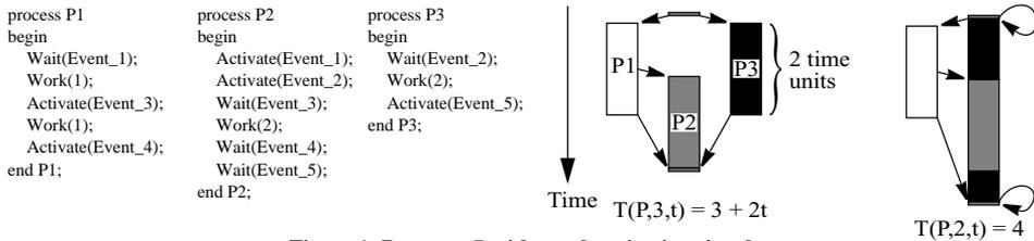
**Figure 1: Program  $P$  with synchronization signals.**
