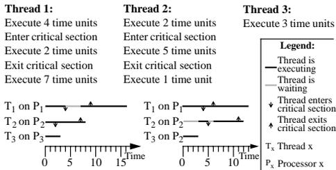
**Figure 2: Illustrating the effect of assigning each thread their own processor. To the upper the three threads are specified. To the lower left the threads are assigned an own processor. To the lower right thread 2 and 3 shares processor 2, while thread 1 is assigned processor 1.**
