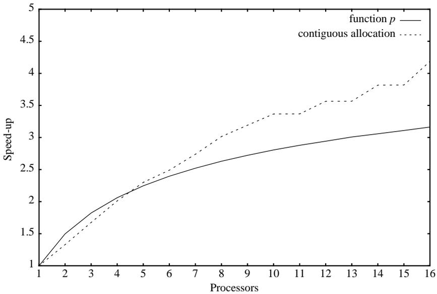
Figure 19: The speed-up for the prime number program on a slow network (latency = 8  $\mu$ s).
