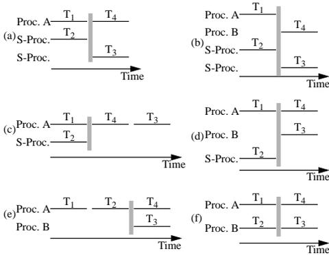
**Figure 4: The different steps in the SGA algorithm for assigning the four threads in Section 3. A shadow processor is named S-Proc. The synchronization is the vertical bar, analogous to a barrier. The final assignment is the one in (f).**
