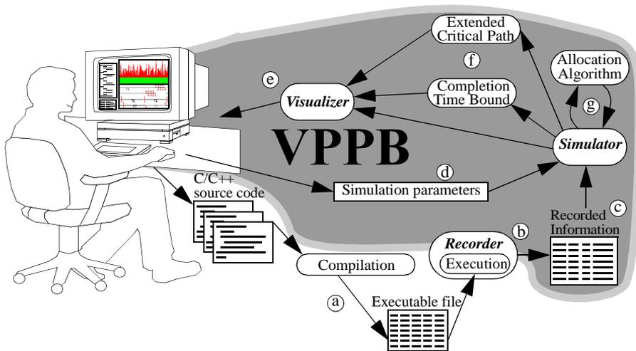
Figure 1: A schematic workflow of the techniques in this thesis.
