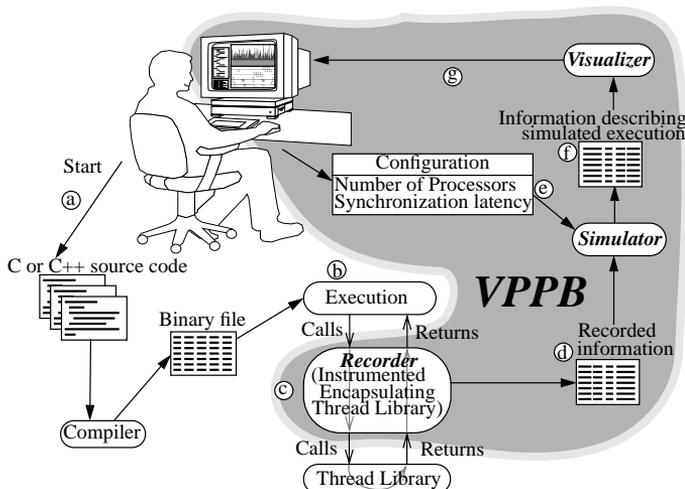
Figure 15: A schematic flowchart of the VPPB system.
