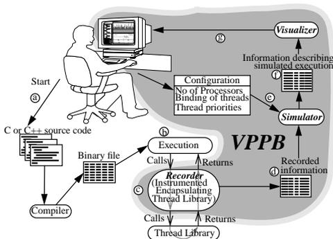
Figure 1: A schematic flowchart of the VPPB system.
