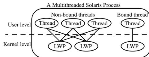
Figure 2: The thread model in Solaris. A bound thread may only execute on the LWP that it is bound to, whereas a non-bound thread may execute on any LWP that is not bound to a user level thread.
