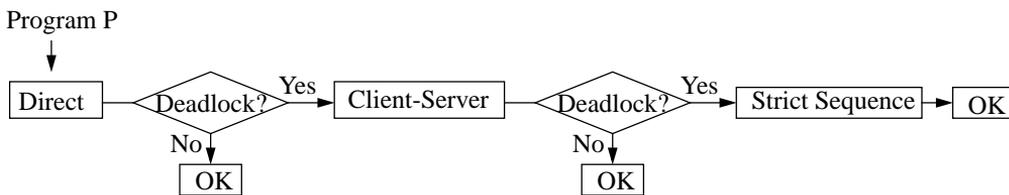
**Figure 14: Practical scheme showing how to use the three simulation models.**
