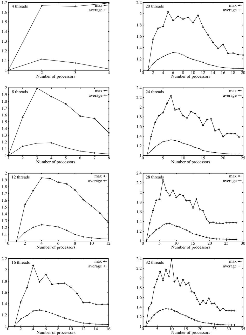
Figure 6: Simulation results for C-SGA. The Y-axis shows (execution time for binpacking) / (execution time for C-SGA).
