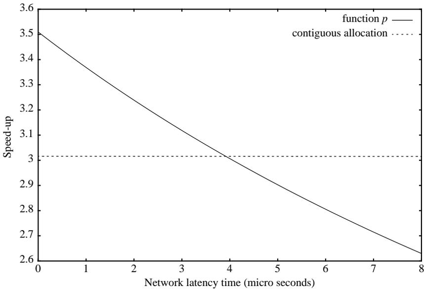
Figure 20: The speed-up for the prime number program on eight processors with various networks latencies.
