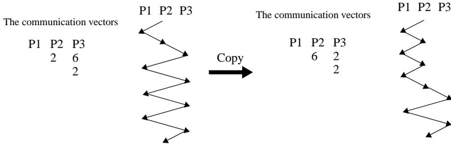
Figure 12: Making a copy where we have swapped the communication frequencies of processes P2 and P3.
