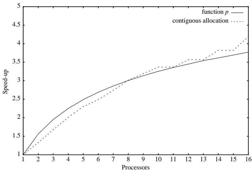
Figure 18: The speed-up for the prime number program on an ordinary network (latency = 4  $\mu$  s).
