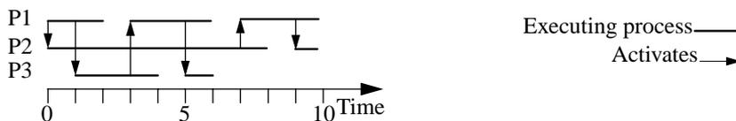
Figure 7: Execution flow of program *Q* when using one processor per process.
