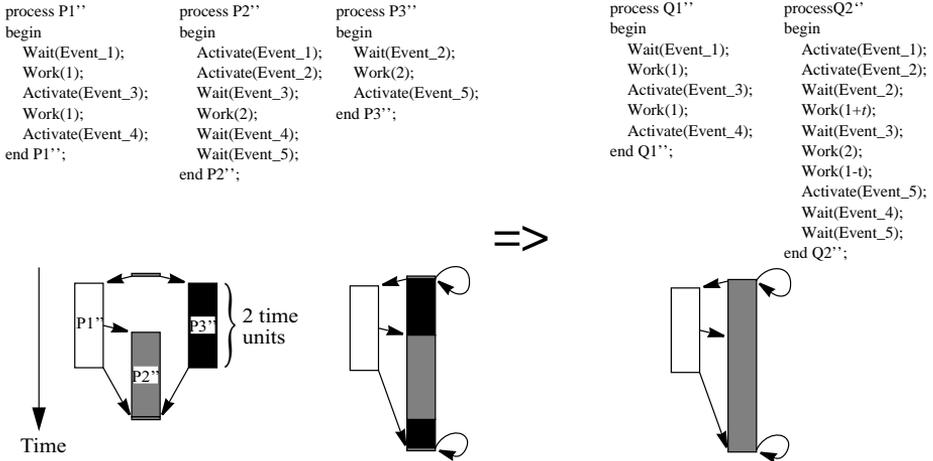
**Figure 6: Transforming a program  $P''$ , allocated to two processors, into a program  $Q''$  with one process per processor.**
