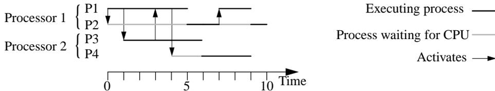
Figure 2: Execution flow of program  $P$  using two processors.
