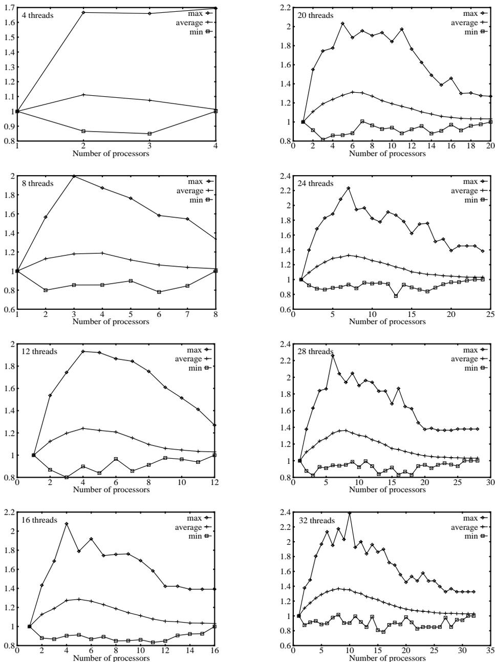
Figure 5: Simulation results for SGA. The Y-axis shows (Binpack execution time)/(SGA execution time).
