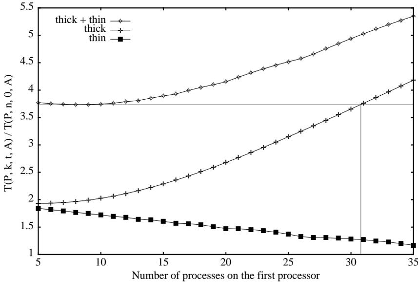
Figure 14: An example showing that the thick part increases and the thin part decreases as the number of processes on the first processor increases.
