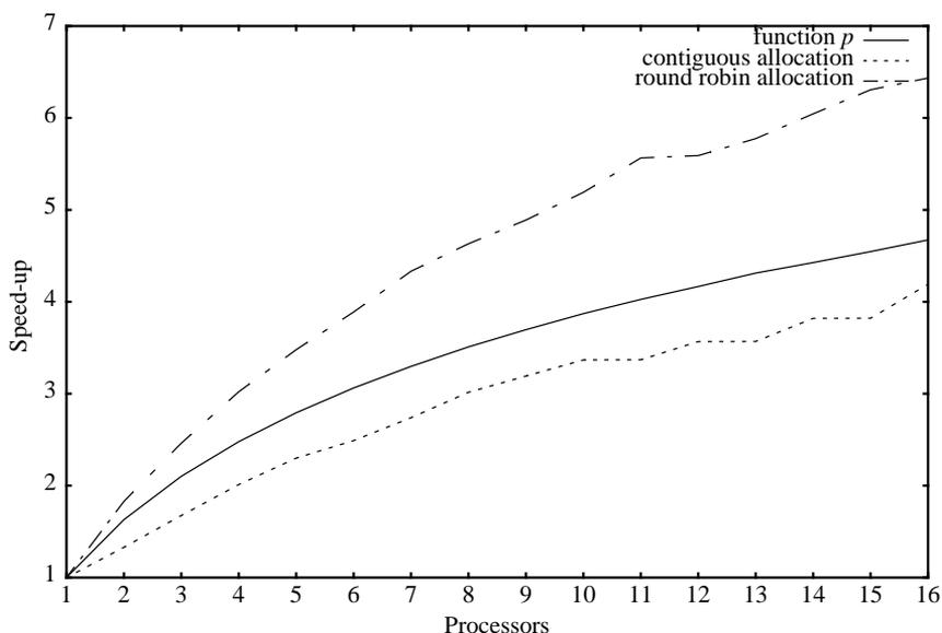
Figure 21: The speed-up using round robin for the prime number program (latency = 0  $\mu$ s).
