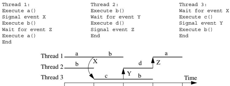
FIG. 1. A simple program with three threads and the execution on a multiprocessor with three processors.
