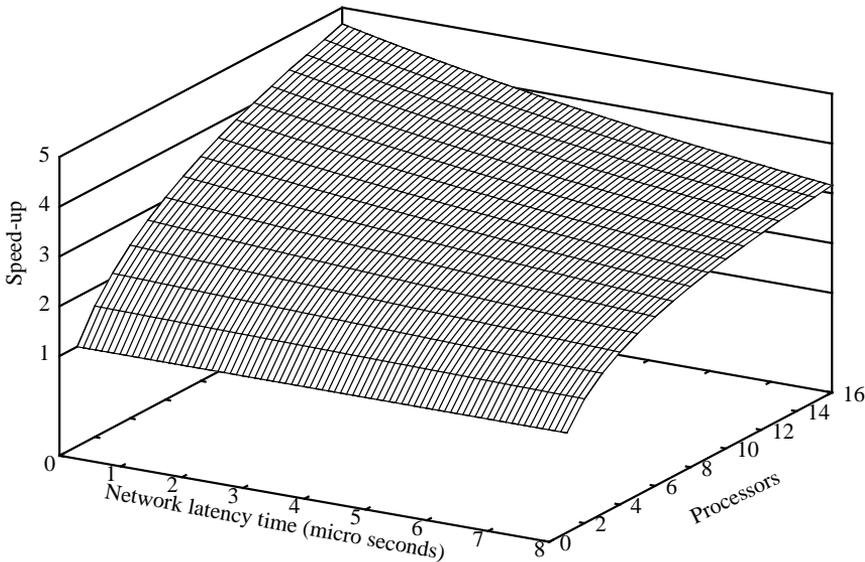
Figure 22: The speed-up for the prime number program by applying function  $p$ , varying number of processors and networks latencies.
