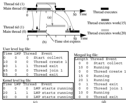
Figure 5: Merging the user and kernel level log files.
