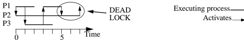
**Figure 5: Execution flow of program  $Q'$  when using one processor per process.**
