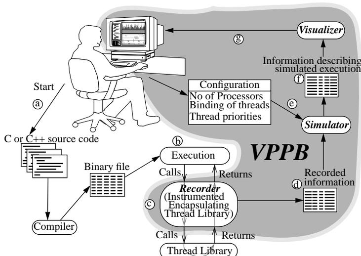
Figure 13: A schematic flowchart of the VPPB system.
