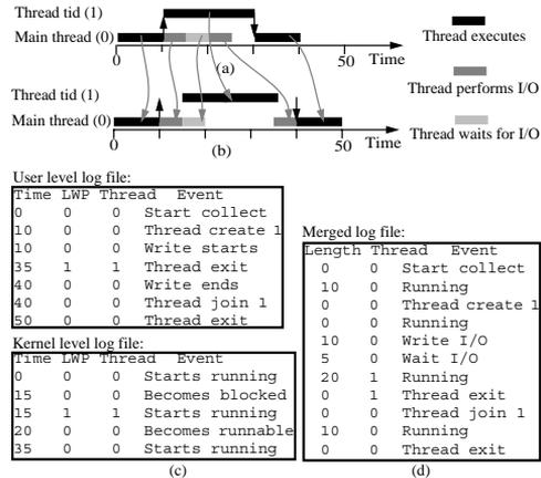
Figure 6: Merging the user and kernel level log files.
